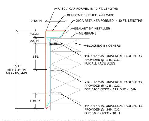
PRE-DRILL WITH 3/16-IN. DRILL BIT FOR MASONRY CONDITIONS.
